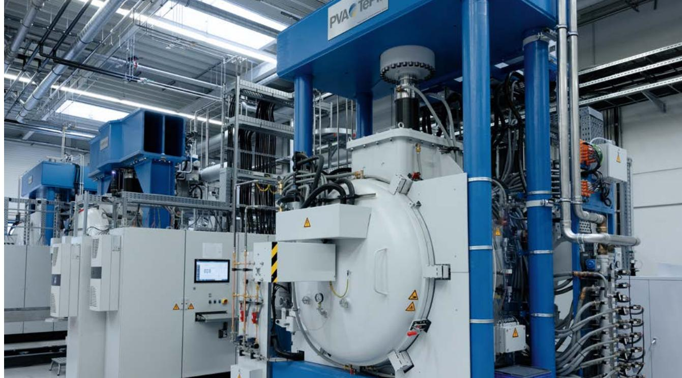
*Under high pressure, individual layers are bonded together into a single structure in this machine.*
