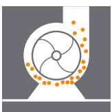
Pump Eccentricity, cavitation
