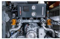
To process the flow, level and RFID data from the field, a CR1058 programmable graphic display for controlling mobile machines has been implemented, which records all the information via the Ethernet/IP protocol, displays it on the screen
