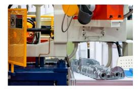
To achieve the lowest possible reject rate, the company must ensure certain process values. Because if defective components are processed to completion without further quality checks, very high costs are incurred in production and a lot of material is wasted on rejects. Defects usually occur due to residues in the die casting moulds or because the vacuum in the mould is insufficient. Residues are caused by incorrect cleaning or application of the release coating;
