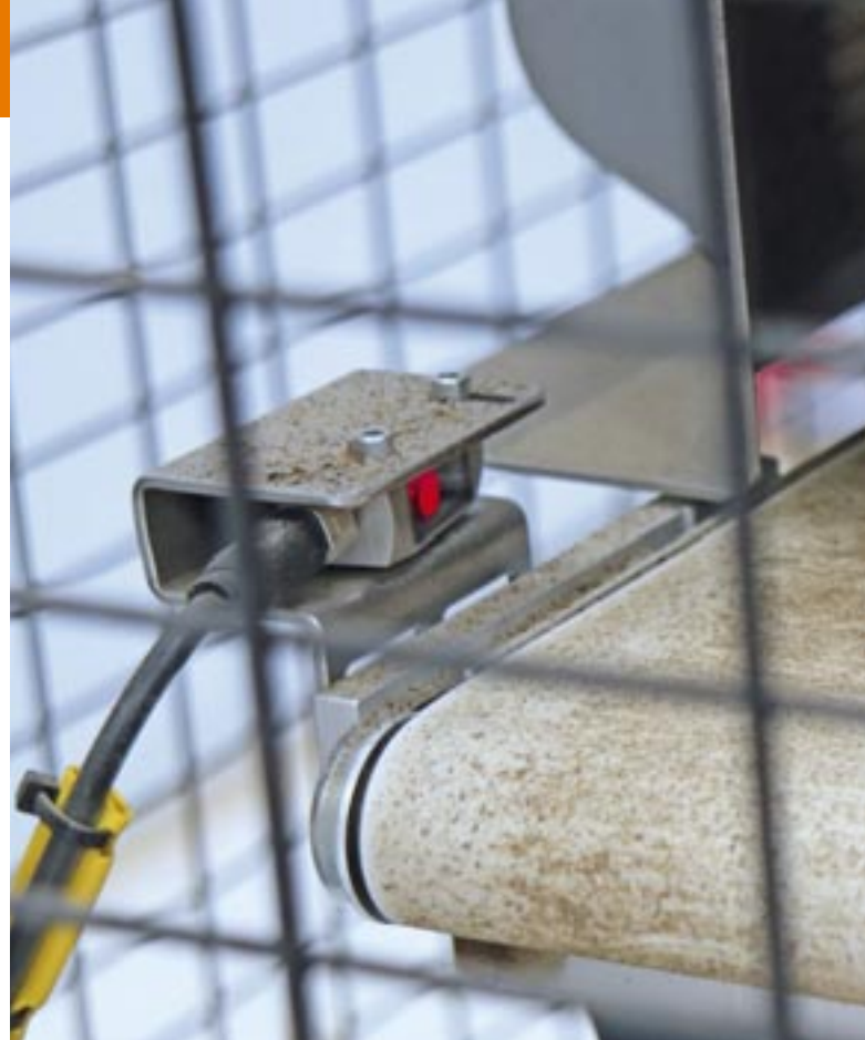
The ifm O6-series diffuse reflection sensors monitor the flow of material.
