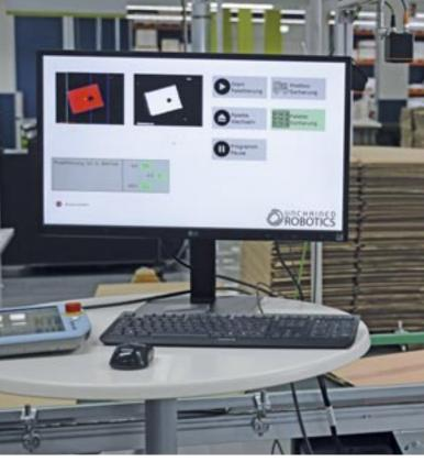
Based on the data transferred by the sensor, the software calculates the robot arm's movements to ensure precise positioning of the package at the placement location.
