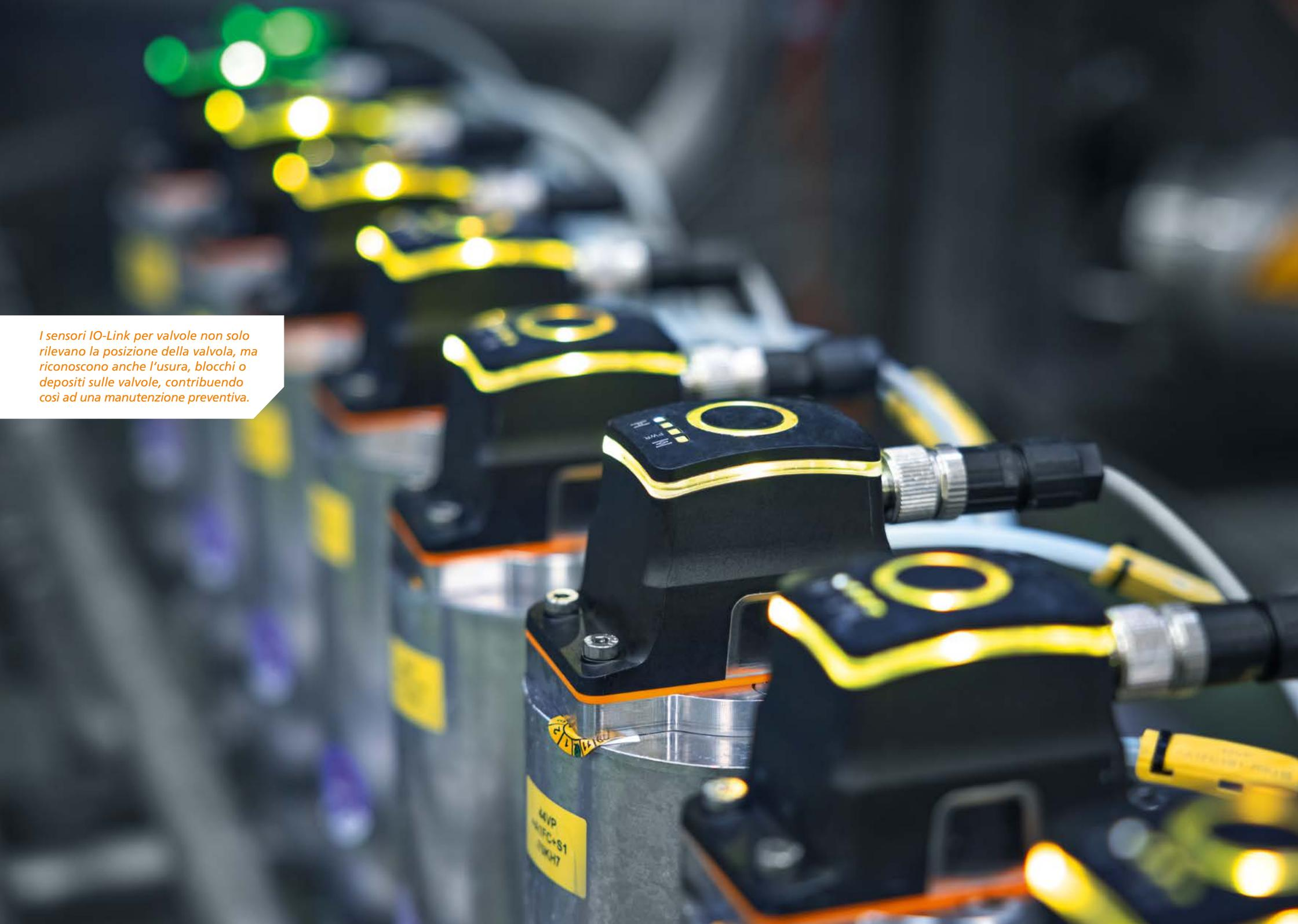
A close-up, perspective view of a row of industrial valves in a factory. Each valve is equipped with a black IO-Link sensor unit. The sensors have a yellow circular logo and a small display with four LEDs. Yellow cables connect the sensors to the valves. The background is blurred, showing more valves and green and yellow lights.
