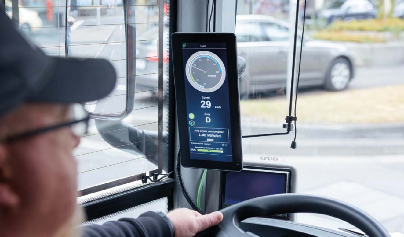
In the cockpit, the robust CR1203 graphic display provides the driver with all key parameters of the electric drive system.
