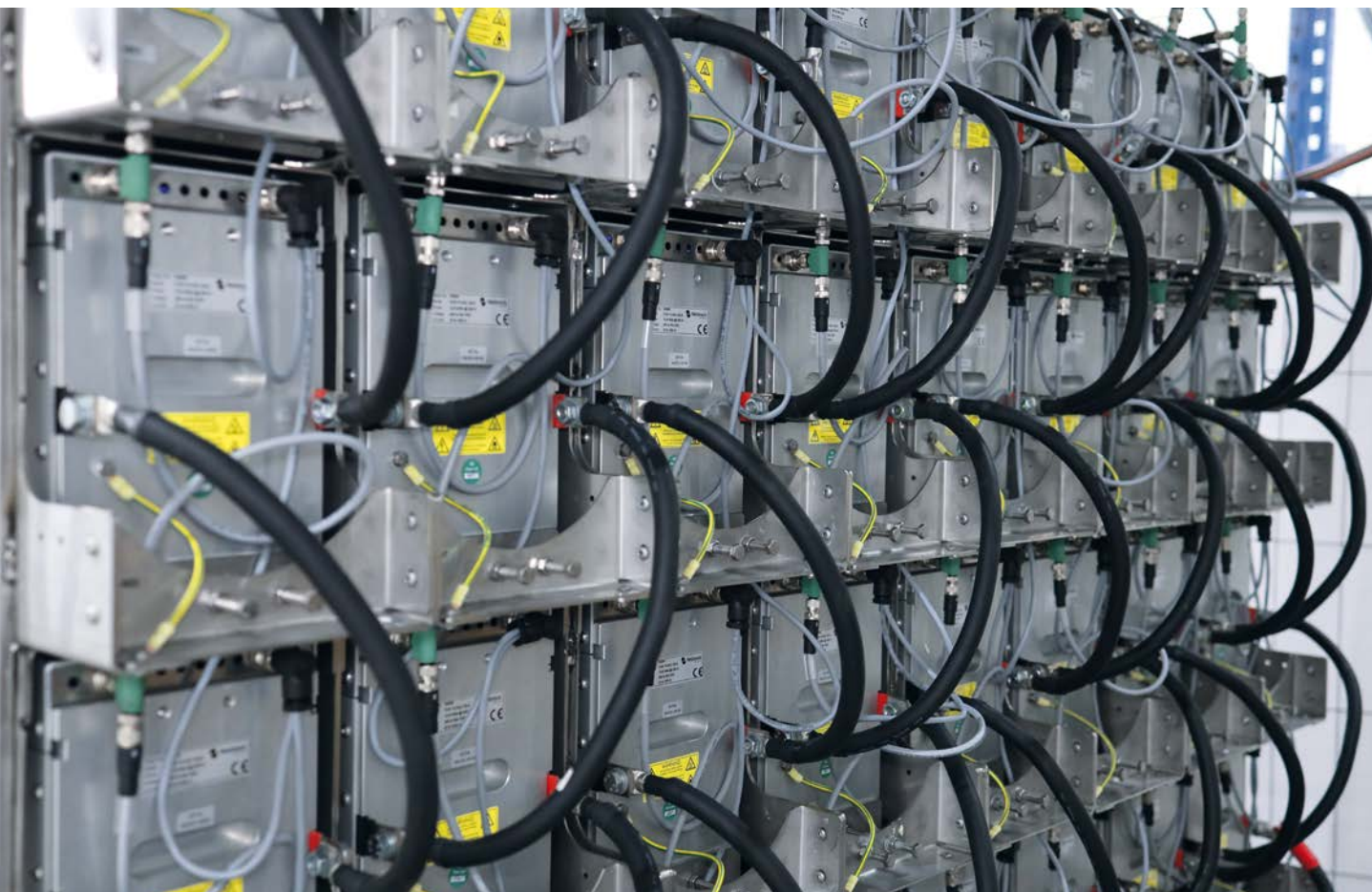
The 32 low-temperature PEM fuel cells produce the energy for propulsion of the vessel.
