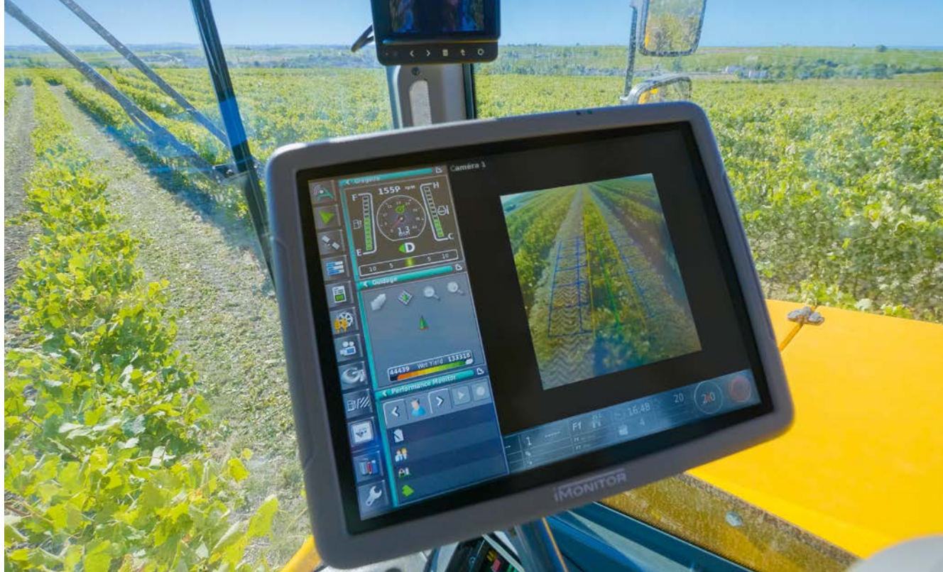
The driver only controls the operating speed, EasyPilot does the steering.
