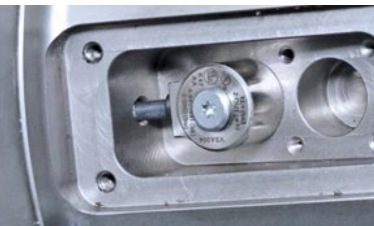
Constantly listening: Vibration sensor VSA004 from ifm placed right on the spindle.
