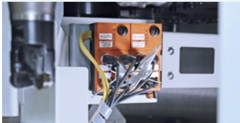
Reduces wiring: AS-i modules collect sensor data and transfer it to the controller via the 2-wired bus cable.
