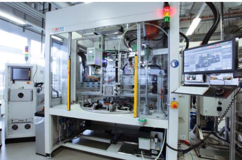
In this system, heat-conductive paste and sealing compound are applied and the product passes through the final joining process.
