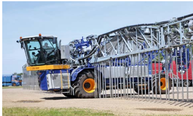
The self-propelled slurry spreader SDS 8000 can spread up to 200 tons of slurry per hour via the hose.
