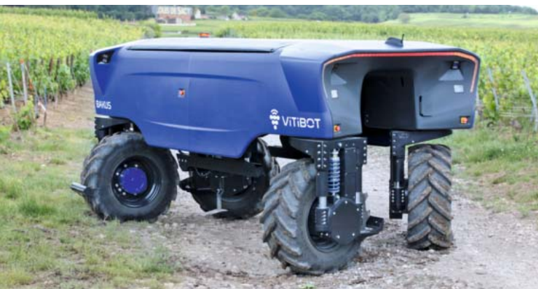
Autonomous turning manoeuvre: thanks to several 3D cameras potential obstacles are avoided and the Vitibot can drive through the rows with the vines perfectly centred below the vehicle.
