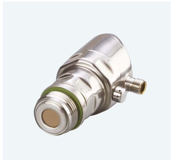
The high-purity ceramic measuring cell is installed flush without dead space and meets the requirements for aseptic applications.
