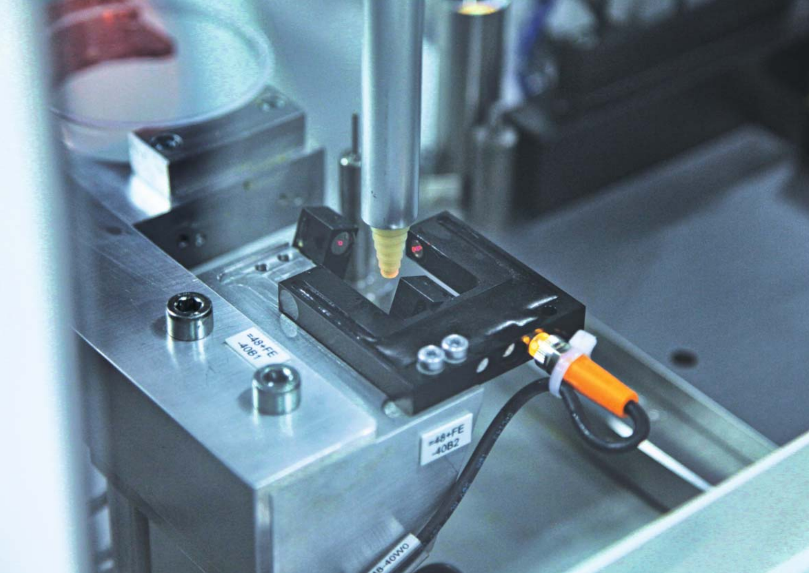
Two photoelectric fork sensors with fine light beam during the reference movement of the fine nozzle.
