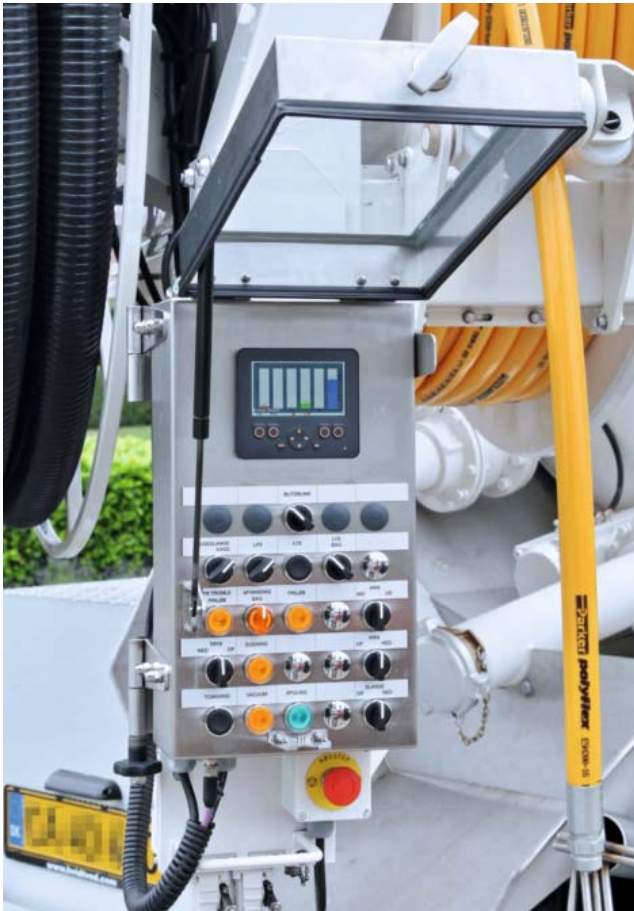
The BasicDisplay CR0451 indicates the most important parameters on the control panel.
