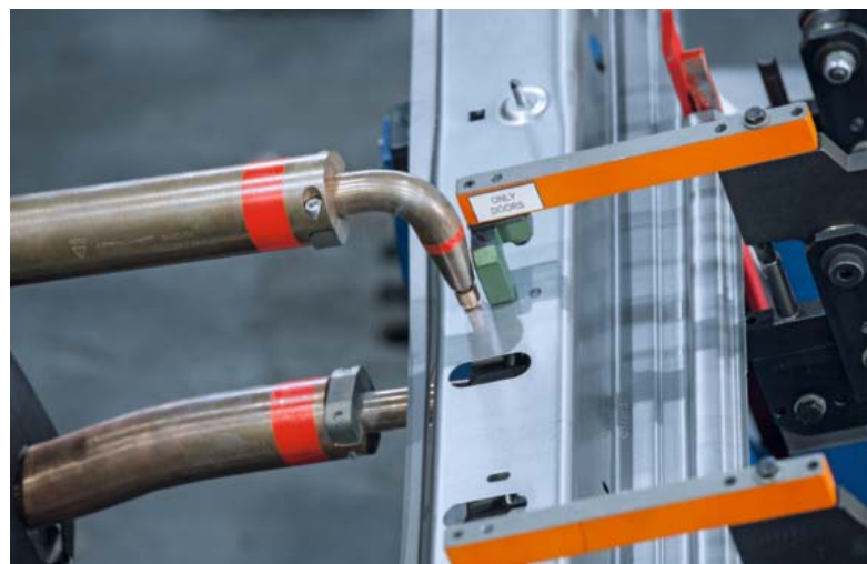
Free installation space: No more sensors are required in the area of the welding tongues and weld spatter.
