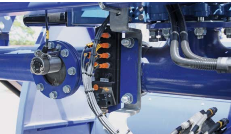
Robust decentralised I/O modules receive sensor signals and transmit them to the PLC via CAN bus.
