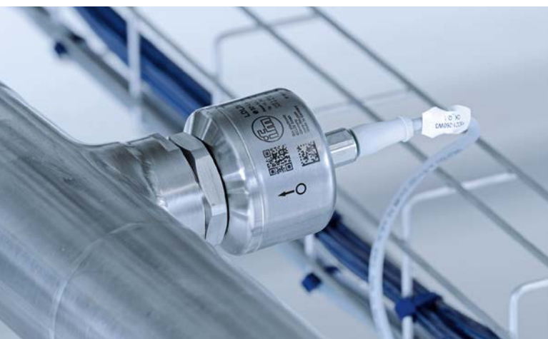
The conductivity sensor LDL200 reliably recognizes if clear water or cleaning detergents from the CIP process are in the lines. Simultaneously it also measures the temperature and transfers both measuring values using IO-Link to the control system.
