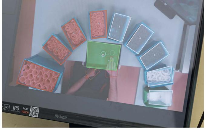
The display guides the worker through the packaging process. The software processes the position, orientation and height of the hand and can thus ensure correct execution of the individual steps. The colour scheme for the worker's visual orientation can be defined as required.
