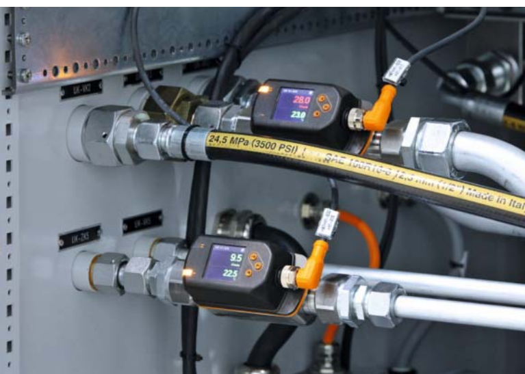
Two measured values (volumetric flow quantity and temperature) with only one sensor.
