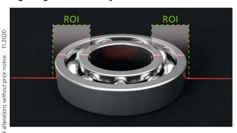
To make the determination of differences between nearly identical components even more reliable, the profile evaluation can be narrowed down to the relevant object area with green markings by using the Region of Interest function.
