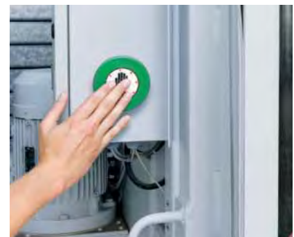
Activation of a process as long as the hand touches the sensor.
