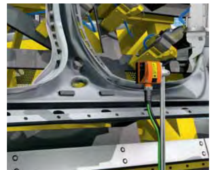
The presence of adhesive pads for noise reduction is checked.
