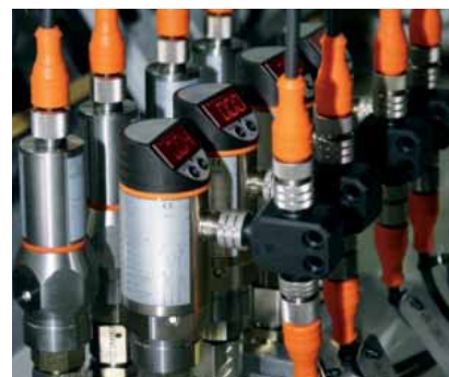
Differential pressure measurement in filter monitoring.
