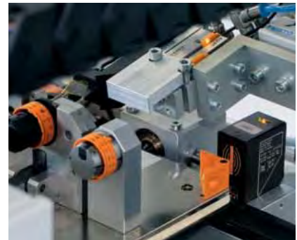
Safe detection of the end positions even for short cylinders.
