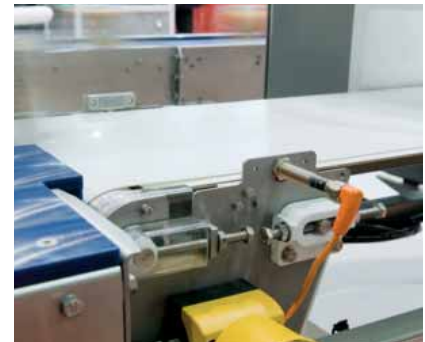
Safe detection of transported parts on a conveyor belt.
