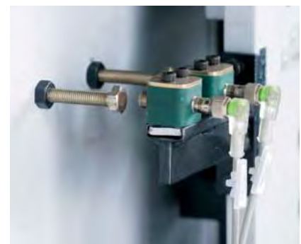
Magnetic sensors provide long sensing ranges.
