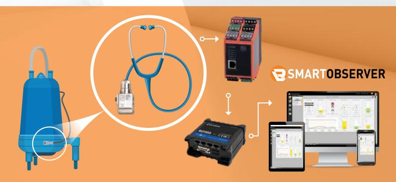
At Lower Murray Water, we have found vibration analysis on our submersible pumps to be very beneficial. The submersible pumps and subsequently the sewer pump station were frequently receiving call-outs due to blockages. The vibration data captured facilitated quicker response time from our maintenance staff and a better understanding of the levels of vibration produced. The ifm technical team were very helpful throughout installation, setting up communications and monitoring the results.
