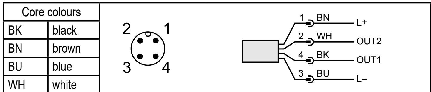
OUT1: switching output or IO-Link
