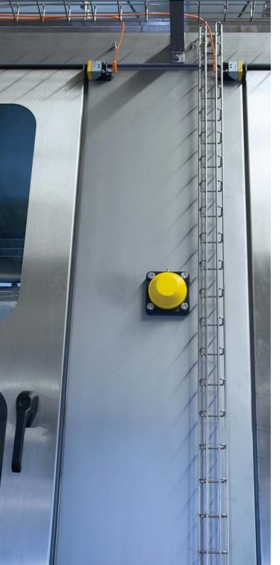
The doors of the system are monitored by fail-safe inductive sensors.
