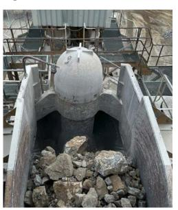
A central process step is monitoring the level in the gyratory crusher. A defined limit value must not be exceeded in order to avoid overfilling, especially as the crusher is continuously fed via a conveyor belt. The harsh, dusty ambient conditions make reliable measurement difficult. Nevertheless, precise level monitoring is essential for smooth and safe operation.
