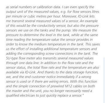
IO-Link supports comprehensive parameter setting. Output functions, measuring ranges, switch points and other parameters can be freely selected within the characteristic values of the sensor. Where many different sensors were required before, one IO-Link unit is often all that is needed today.
