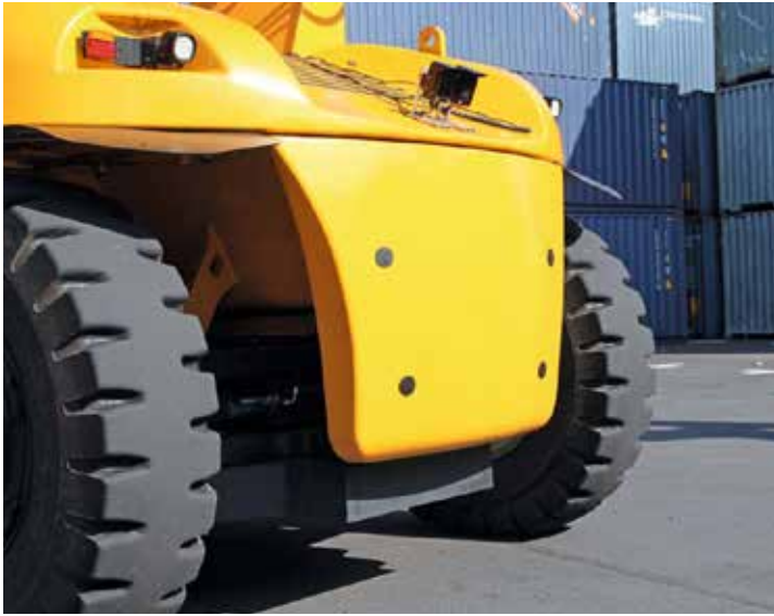
Automatic collision avoidance: 3D camera at the rear automatically warns of obstacles and possible collisions.
