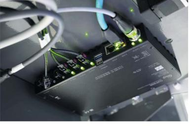
The Video Processing Unit is the central component of the O3R system. It offers the possibility of connecting up to 6 cameras.
