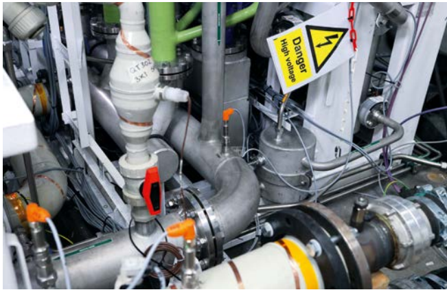
Precise continuous monitoring of pressure, level and temperature values is necessary to ensure efficient operation of the hydrogen propulsion system.
