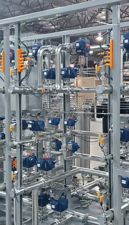
Instead of routing the cables of all sensors of the filtration system to a central controller, IO-Link masters receive the data in a decentralised manner and forward it as a bundled package. This reduces cable routes, saves time and eliminates sources of error.
