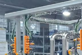
The IO-Link masters receive the data from the sensors in a decentralised manner and forward it as a bundled package. This reduces cable routes, saves time and eliminates sources of error.
