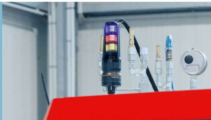
The IO-Link-based LED light tower is clearly visible from a distance and features an integrated buzzer.
