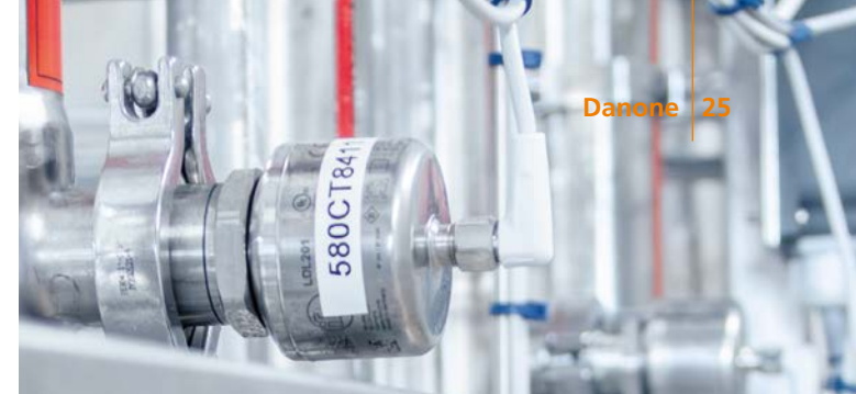
The LDL200 conductivity sensor ensures the correct, efficient execution of the CIP process.
