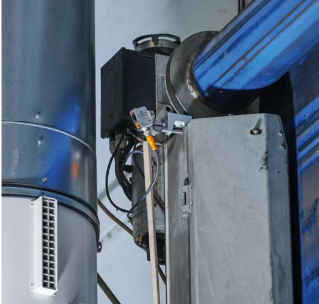
A photoelectric sensor checks whether the door is open or closed.
