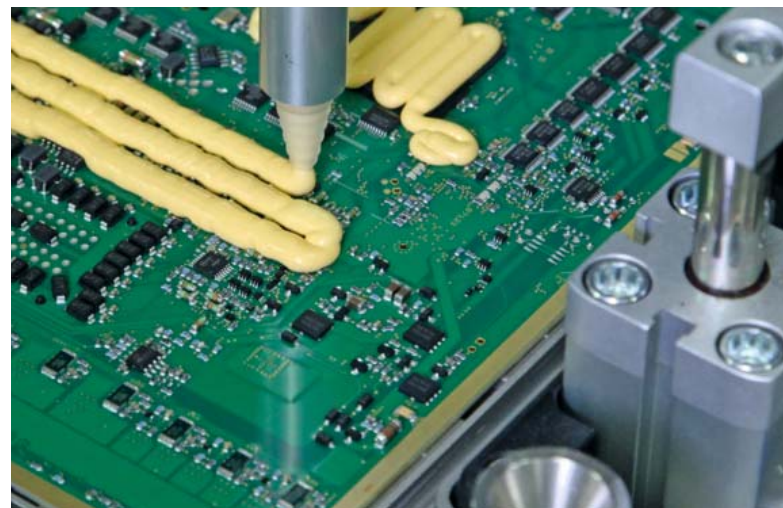
Application of the 2-component heat-conductive paste onto the PCB.
