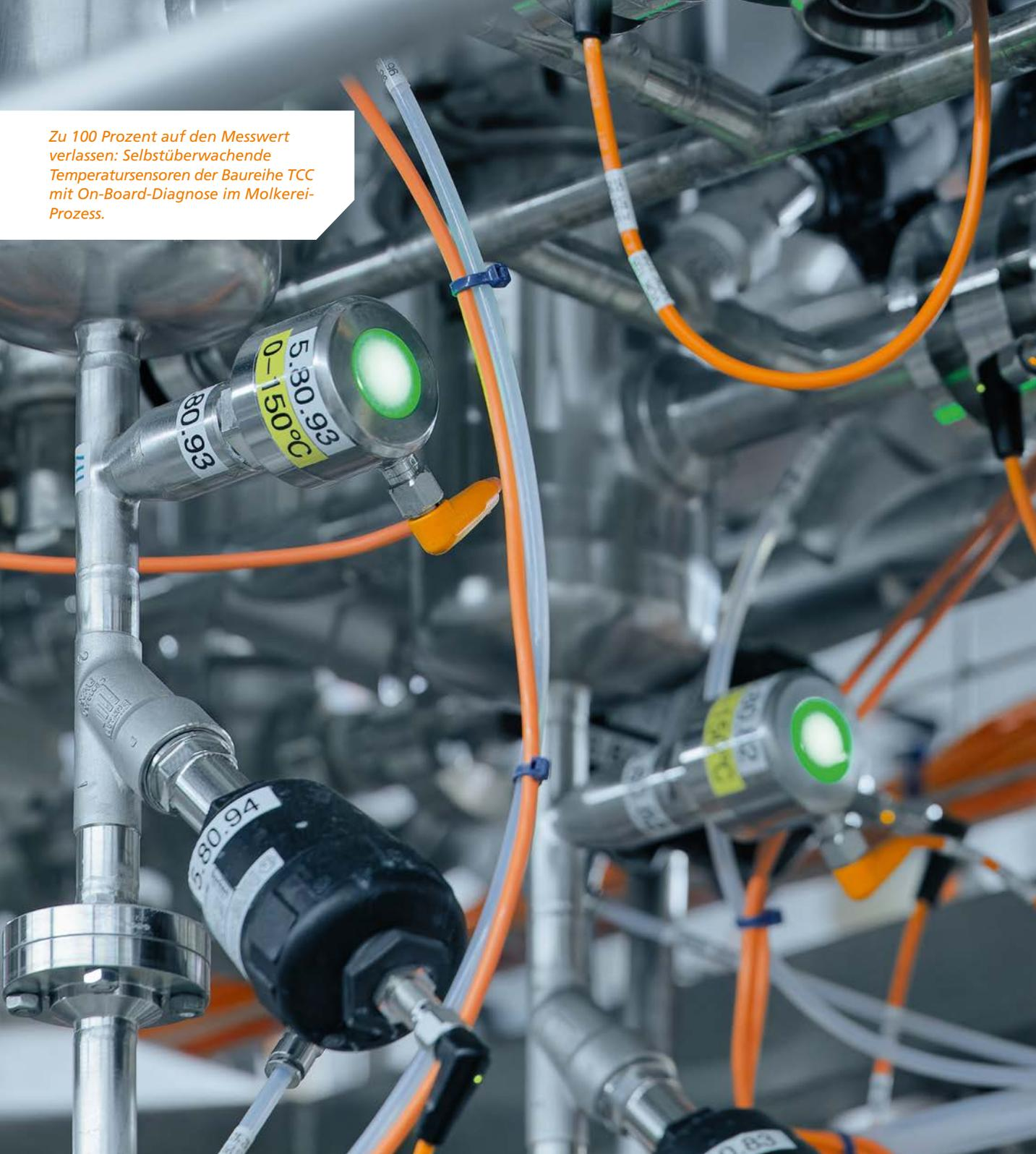
The image shows a close-up of industrial machinery, likely a milk processing plant. Several temperature sensors (TCC) are mounted on metal pipes. The sensors are cylindrical with a green LED light on top. One sensor in the foreground has a yellow label with the text '5.80.93' and '0-150°C'. Another sensor below it has a black label with '5.80.94'. Orange cables are connected to the sensors. The background is a complex network of metal pipes and machinery.
