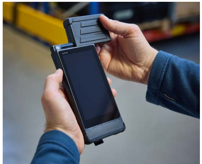
The various antenna modules on the handheld device's top edge can easily be replaced.
