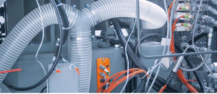
The sensor data from the recycling plant is collected decentrally via an IO-Link master and forwarded to the control system in bundled form.
