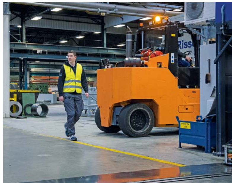
Persons behind the forklift truck are difficult to see for the driver. The anti-collision system helps to avoid critical situations when reversing.
