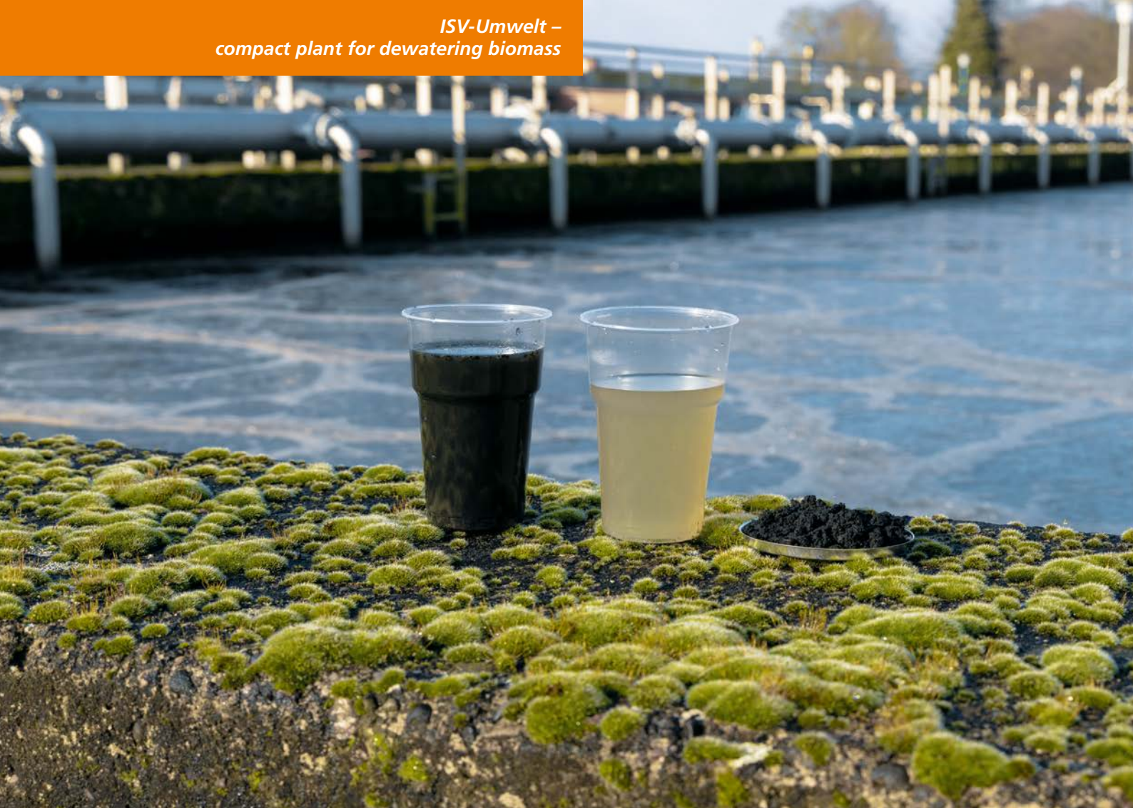
The sewage sludge (left) is separated into water (centre) and dry substrate (on the tray on the right).
