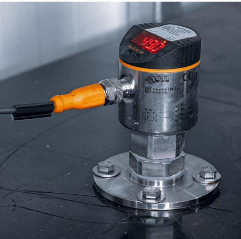
The LR7000 level sensor uses a microwave to detect the level in the flocculant preparation tank.
