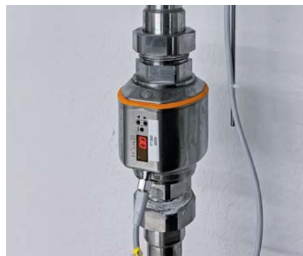
The flow sensor transmits several measured values to the control system via IO-Link.
