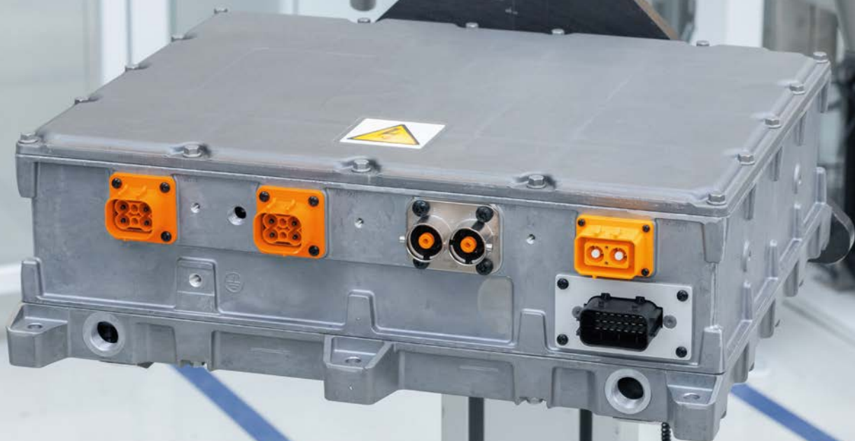
The finally assembled ED3 onboard charger.
