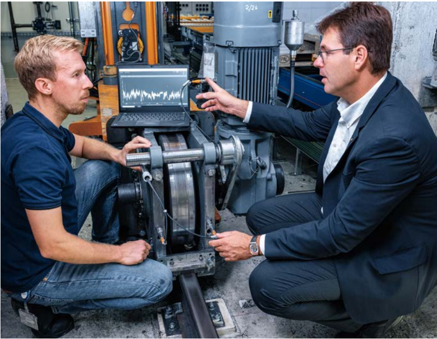
The diagnostic software moneo interprets vibration data and alerts the team in case of anomalies, supporting on-site adjustment and alignment.
