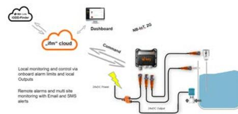
As only small amounts of data are transmitted, such narrowband networks are completely sufficient. Via an IO-Link input module, the io-key in the pumping station is connected to the analogue sensor signals of the level sensors and the signals for the status of the pumps. The installation is based on the plug & play principle: After connecting the sensors to the io-key,
