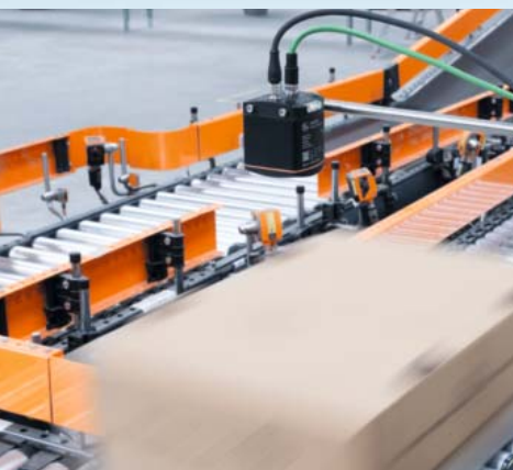
Heavy weight in logistics: 3D sensors measure packages to calculate the dimensional weight.
