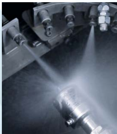
Ingress-resistant under extreme conditions: test for the IP 69K protection rating.
