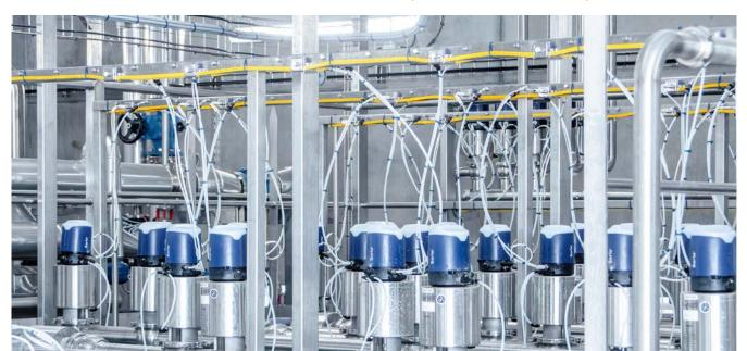
The striking yellow AS-i flat cable runs through the entire process chain. The information from Definox's Sorio valve control heads is also transmitted seamlessly.
