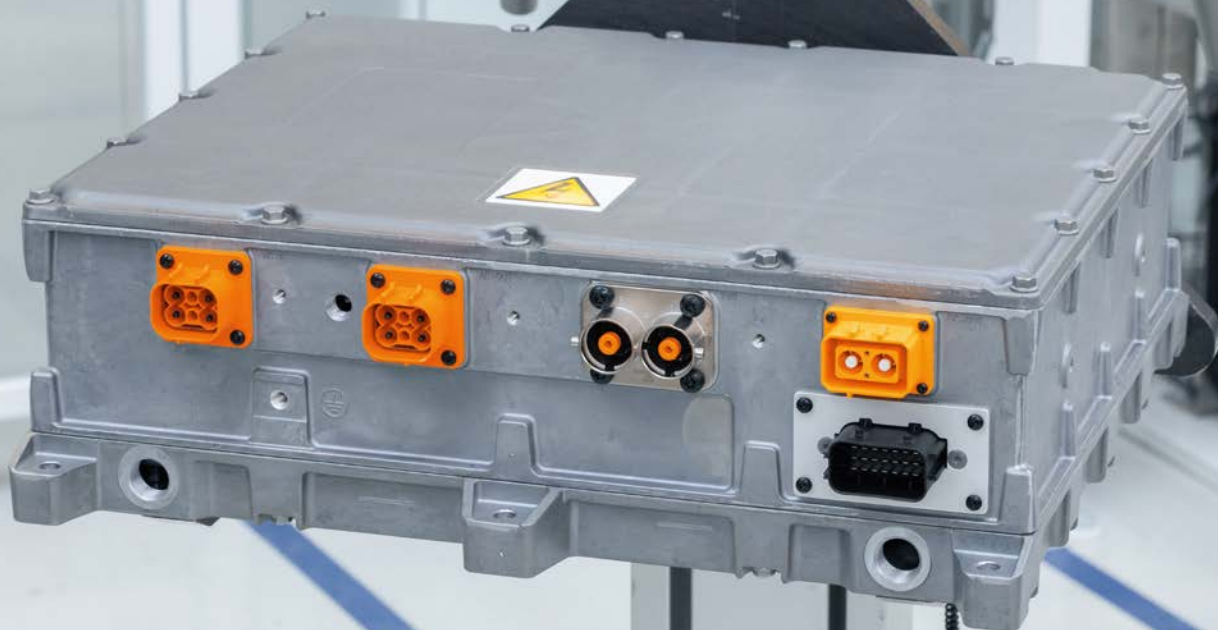
The finally assembled ED3 onboard charger.
