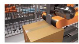
process is central to a reliable logistics workflow: when errors occur at this stage, the plant comes to a standstill or the products in the parcels can be damaged. Conventional photoelectric sensors often fail to reliably detect the transparent and reflective adhesive strips in the machines. As a result, correct parcel sealing had to be checked manually up to now.
