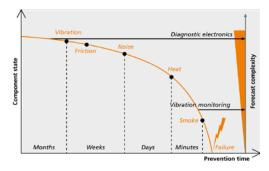
of problems. Unbalances may occur in drum bearings, gears and hoist motors. If the affected parts fail, the result is a plant standstill, which is often associated with high costs. By using sensor technology, however, these problems can be counteracted at an early stage.
