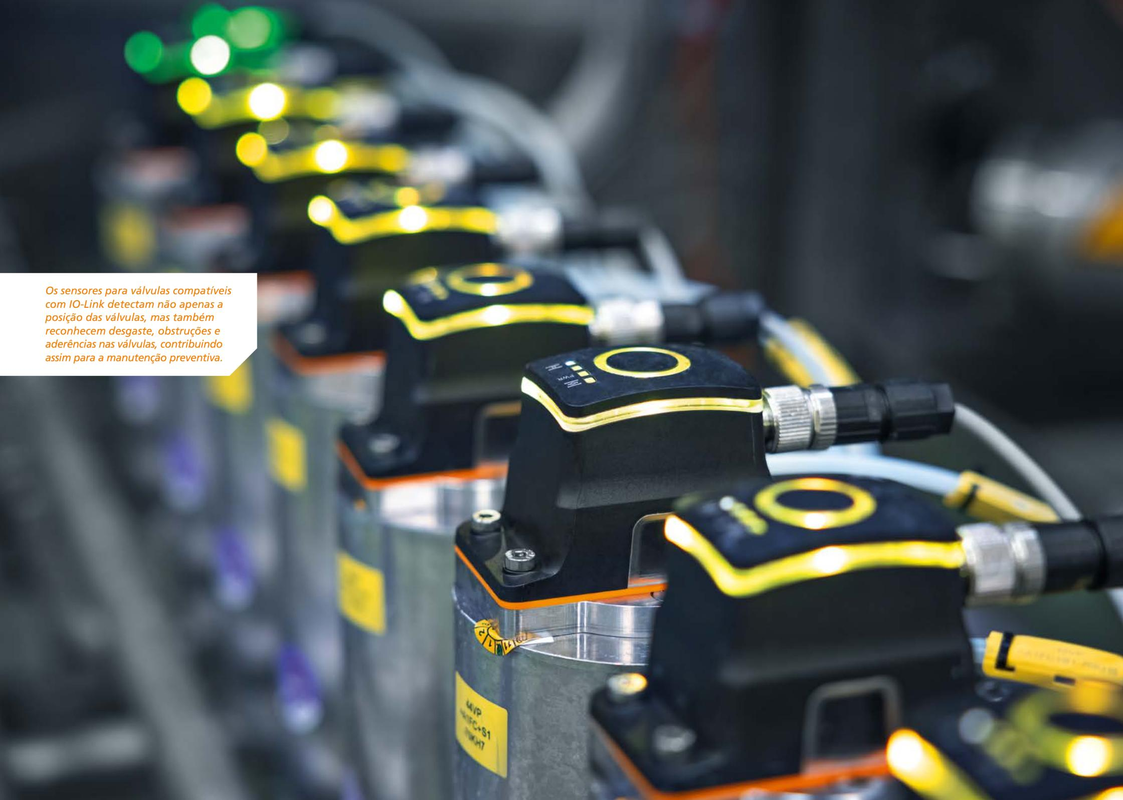
A close-up, perspective view of a row of industrial valves in a factory. Each valve is equipped with a black IO-Link sensor unit. The sensors have a yellow circular logo and a small display with four LEDs. Yellow cables connect the sensors to the valves. The background is blurred, showing more valves and factory lights.
