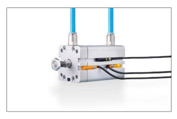
One sensor instead of two: On short-stroke cylinders, one IO-Link cylinder sensor (upper groove) is now sufficient to detect both end positions instead of two conventional sensors (lower groove) as was previously the case.
