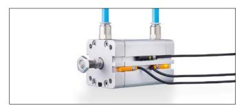
**One sensor instead of two:** On short-stroke cylinders, one IO-Link cylinder sensor (upper groove) is now sufficient to detect both end positions instead of two conventional sensors (lower groove) as was previously the case.
