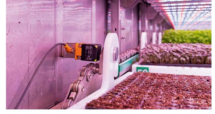
Inductive sensors from ifm ensure safe and reliable transport processes in the ModuleX.
