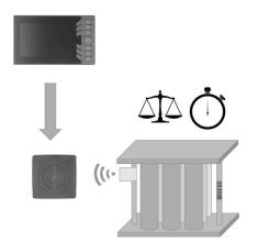
After that, the unit is weighed and the result serves as a baseline for later production steps and to verify again that the correct number of cells are present. This weight information is tied to the unique identifier within the database. Efficiency of the cell is tracked by enter/exit time.
