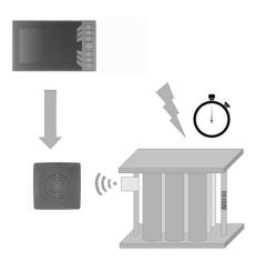
The unit is placed in a voltage testing machine to ensure that it has been assembled correctly according to the final build instructions. To track the efficiency of the line, the time within the testing cell is monitored, and the results of the test are tied to the UHF identifier for later traceability.
