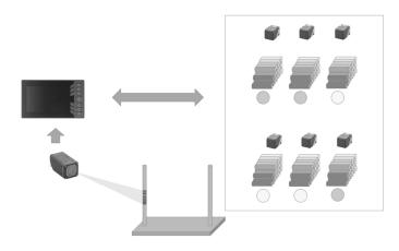
After voltage testing, the cells are separated into serialized production batches. The batches must retain the manufacturer and lot information through the production process. To achieve this, the bins are tracked with HF RFID, enabling a pick-to-light system for the assembler based on the presented work order.
