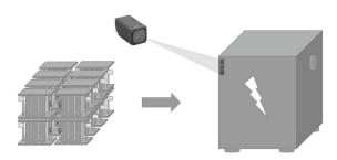
Following the pack creation, and a subsequent voltage check on the unit as a whole to ensure proper operation, a cover is placed on the entire pack, which contains a unique barcode for tracking throughout the warehouse and in the future.
