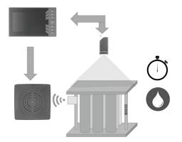
The module then moves to the adhesive cell – time is critical here and is tracked for each step. An inspection camera verifies the positive/negative side of each module. Each of them has independent adhesive gluing patterns. Time of enter and completion is tracked to ensure that the epoxy received the correct treatment.
