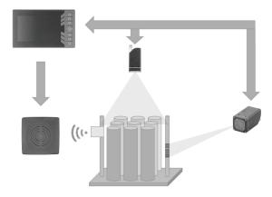
The code read initializes the correct inspection program. Upon passed inspection, the barcode identification is written to the UHF RFID tag. The UHF tag will be used in all future assembly steps as the engraved code rotates until assembled into the pack and no longer reliable.
