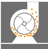
Pump Eccentricity, cavitation
