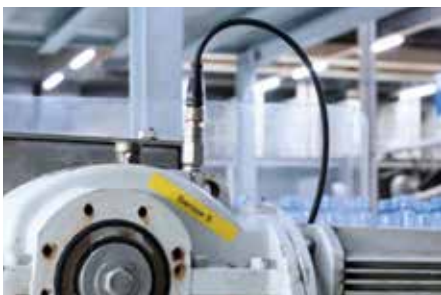
Vibration sensors on the drives detect even smallest vibrations.
