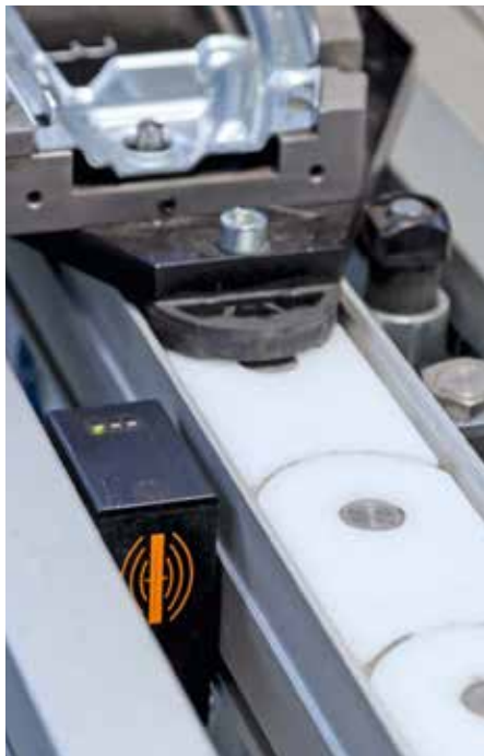
The ID tag chip is installed at the base of the workpiece carrier. The chip can store up to 224 bits.
