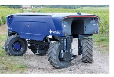
Autonomous turning manoeuvre: thanks to several 3D cameras potential obstacles are avoided and the Vitibot can drive through the rows with the vines perfectly centred below the vehicle.
