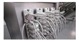
"Harsh" operating conditions in foodproduction due to cleaning processes using high pressure and chemicals often push IO modules to their limits. As a number of manufacturers cannot meet the required IP protection class, an additional control cabinet is required to protect the technology. This renders the solution both more complex and expensive.
