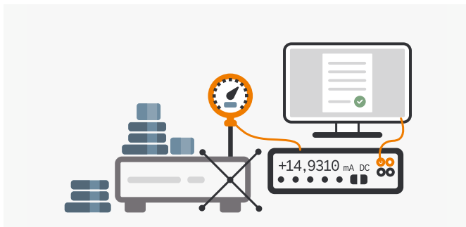
Calibration of pressure gauges by using pressure compensators
